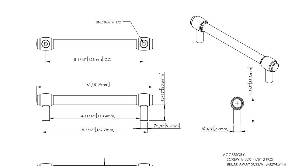
BREAK AWAY SCREW: 8-32X45mm 2 PCS ALL SCREW MATERIAL: STEEL-SAE1006
